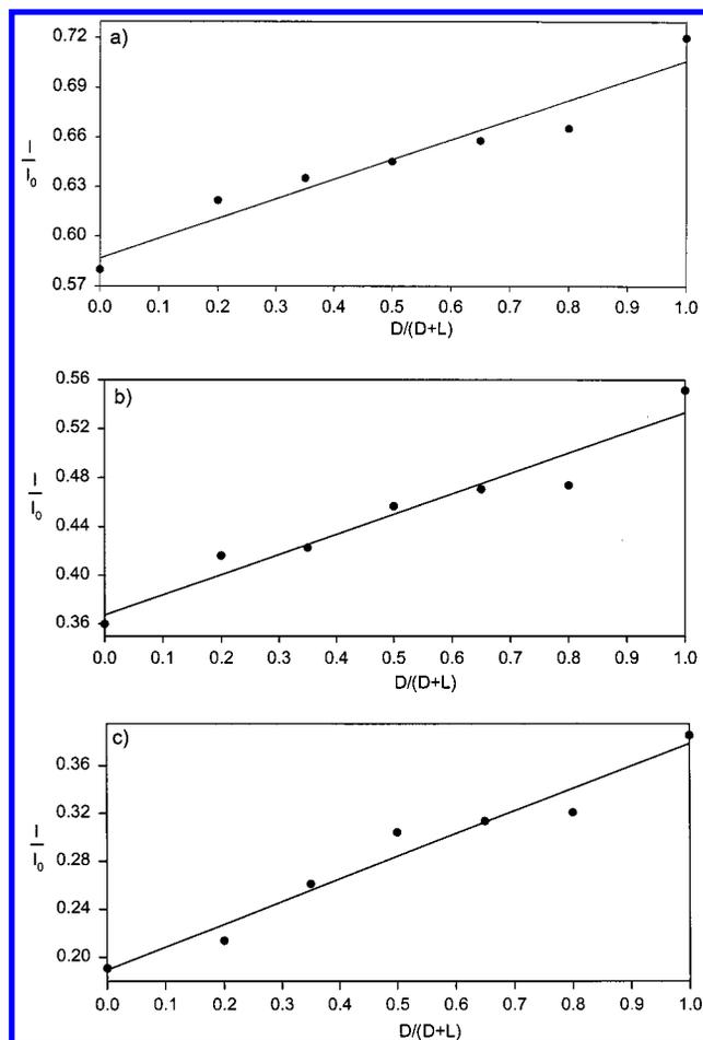
Figure 4. Calibration curve for mixtures of L- and D-alanine at reaction times of (a) 4, (b) 5.5, and (c) 7.5 s. The corresponding complexes are reacted with *n*-propylamine ( $3.0 \times 10^{-7}$  Torr). The points become more linear at longer reaction times.
