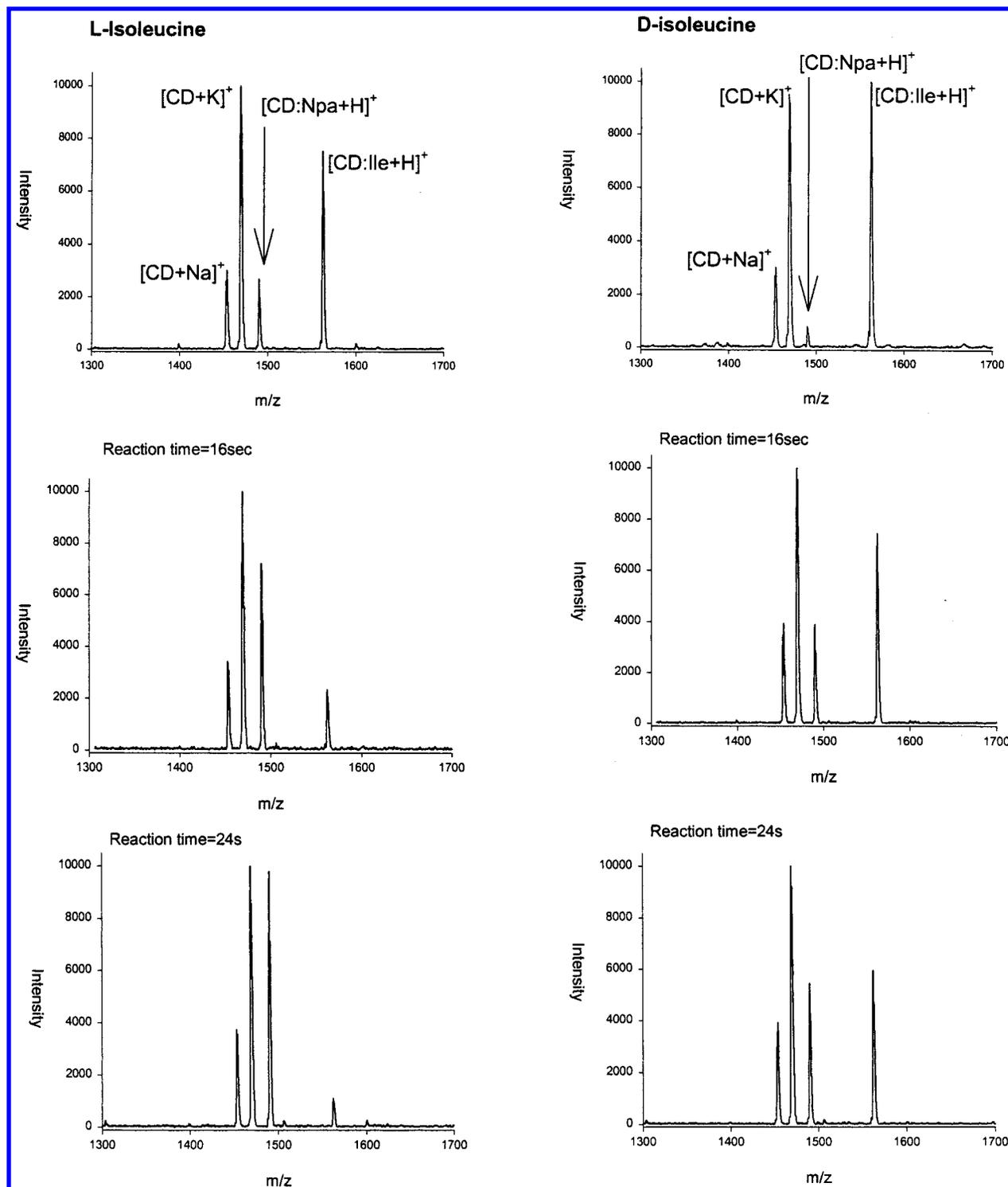
Figure 1. FTMS spectra of enantiomers of protonated isoleucine complexed to  $\beta$ -cyclodextrin (CD) and allowed to react with *n*-propylamine (Npa,  $3.4 \times 10^{-7}$  Torr) for 5 s. The L enantiomer is more reactive than the D as illustrated by the intensity of the product peak  $[\text{CD:Npa+H}]^+$  relative to the reactant peak  $[\text{CD:Ile+H}]^+$ .
