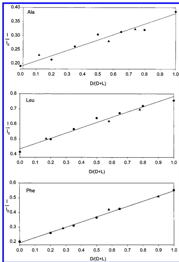
Figure 5. Calibration curves with test mixtures (solid triangles) for Ala, Leu, and Phe. The  $r^2$  values for the calibration curves, without the test mixtures, are 0.961, 0.975, and 0.998, respectively. The test mixtures were analyzed with fresh solutions several days, weeks, and in some cases months after the calibration curves were produced.
