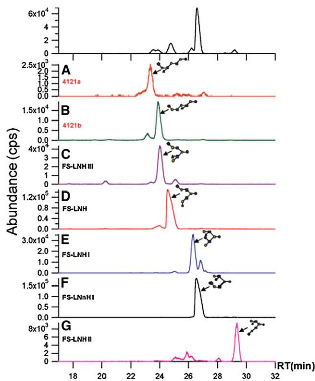
**Figure 1** Separation of isomers of reduced FS-LNH using nanoliquid chromatography porous graphitic carbon chip time-of-flight MS. RT, retention time; FS-LNH, fucosyl-lacto-N-hexaose. Reprinted from Reference (7) with permission.
