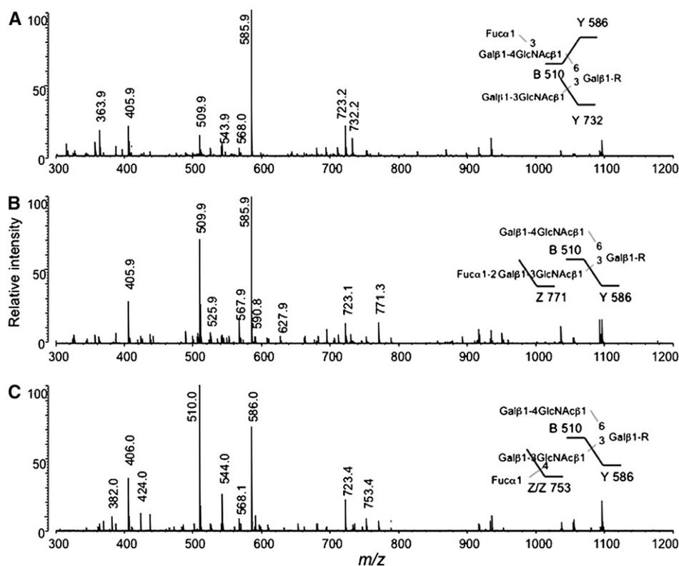
**Figure 4** Differentiation of 3 fucosylated human milk oligosaccharides (HMO) using collision-induced dissociation fragmentation of deprotonated species in the negative ionization mode. MS<sup>3</sup> fragmentation spectra of *m/z* 1079 for the 3 fucosylated HMO (A–C) are depicted together with fragmentation patterns explaining the most important ions. Reprinted from Reference (56) with permission.
