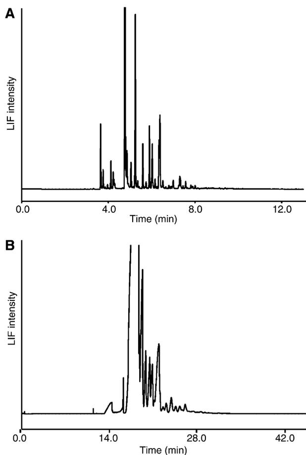
**Figure 2** Separation of 8-aminopyrene-1,3,6-trisulfonic acid–labeled human milk oligosaccharides using capillary electrophoresis with laser-induced fluorescence (LIF) (A) and capillary electrophoresis with LIF MS (B). The adjustments needed for hyphenation with MS result in reduced resolving power and longer analysis times. MS, however, facilitates direct identification. Reprinted from Reference (47) with permission.
