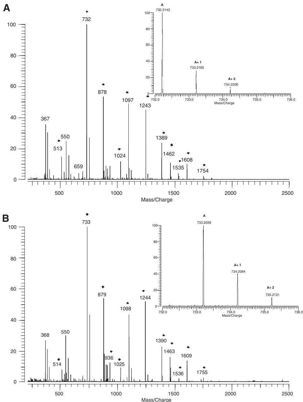
Fig. 3. MALDI-FTICR (+) mass spectra obtained from undeuterated HMOs (A) and deuterated HMOs (B) remaining in medium after inoculation with *E. coli*. The insets show the  $^{13}\text{C}$  isotope distributions at signals  $m/z$  732.3 (A) and 733.3 (B).
